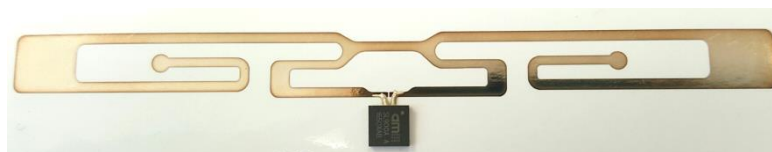
Figure 4: Example of inkjet printed UHF RFID tag design based on AD-224 tag from Avery Dennison with SL900A IC assembled for readout of temperature and other sensor values.
