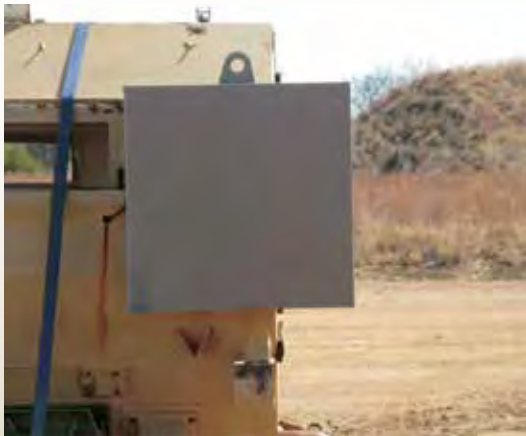
An add-on protection package is tested at the CSIR's detonics, ballistics and explosives laboratory.
