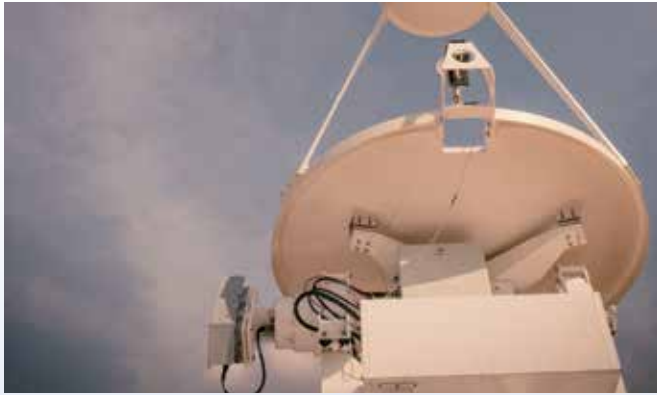
Field trials performed using a mobile, integrated dynamic radar cross-section measurement facility.
