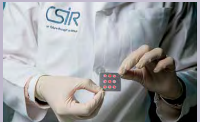
A wax-printed paper-based microfluidic device. Reactions implemented on the device result in a colour change.
