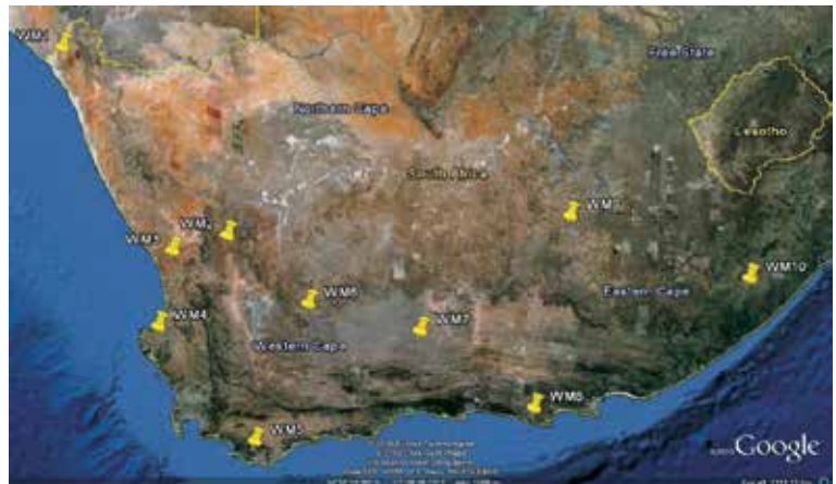
Figure 2: Location of measurement sites within the project domain. The project required three years of measurement data from the ten measurement sites for the verification. Each site consisted of a 60 m mast with anemometry at 62 m, 60 m, 40 m, 20 m and 10 m as well as other meteorological sensors. The data from the sites were sent to the CSIR where it was quality controlled and made available on the WASA web site.
