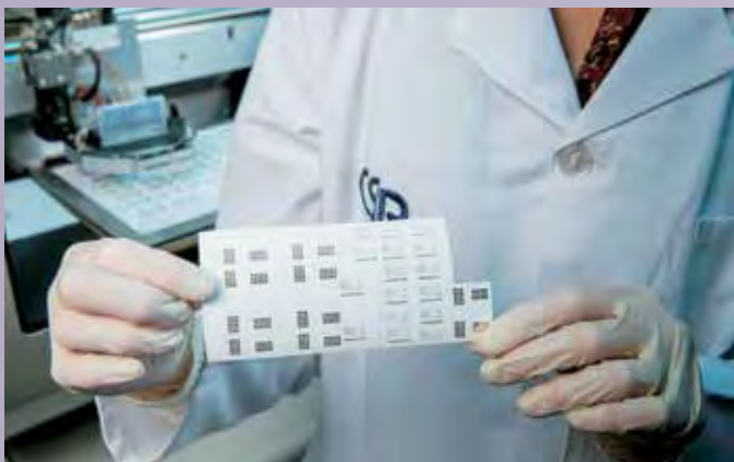
Examples of silver inkjet-printed paper-based sensing electrodes.
