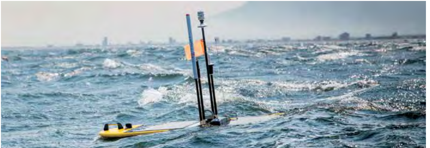
Top: A long-range autonomous iRobot Seaglider. Middle and bottom: A wave glider, pictured off the Western Cape coast between Dassen and Robben Islands with an acoustic echo sounder to determine fish stock levels.
