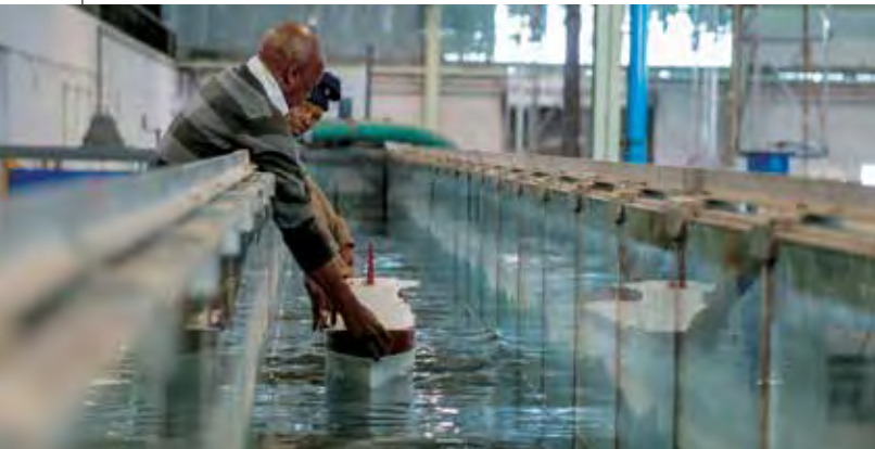
Two of the technologies pioneered at the CSIR hydraulics laboratory are the Keofloat system, where the movement of small lightweight floats (seen top right) are studied to measure the effects of long waves on ships and the Armour Track System, that combines high-resolution images from mounted cameras (opposite page) with laser scanning data of physical models such as breakwater units to track the movement of physical models. The CSIR's Kishan Tuli (left) at work during extensive tests on a detailed model of the Richards Bay breakwater.
