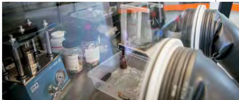
A glovebox used for battery assembling. With this process, work is done inside the machine, protecting the cells from any harmful factors.
