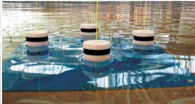
Two of the technologies pioneered at the CSIR hydraulics laboratory are the Keofloat system, where the movement of small lightweight floats (seen top right) are studied to measure the effects of long waves on ships and the Armour Track System, that combines high-resolution images from mounted cameras (opposite page) with laser scanning data of physical models such as breakwater units to track the movement of physical models. The CSIR's Kishan Tuli (left) at work during extensive tests on a detailed model of the Richards Bay breakwater.
