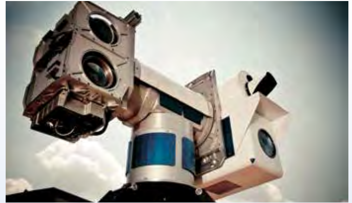
A stand-alone tracker incorporating a multi-spectral high-resolution digital sensor suite that tracks potential threats, and simulates the ocean's movement (or motion) to allow the evaluation of the sensor suite on land.
