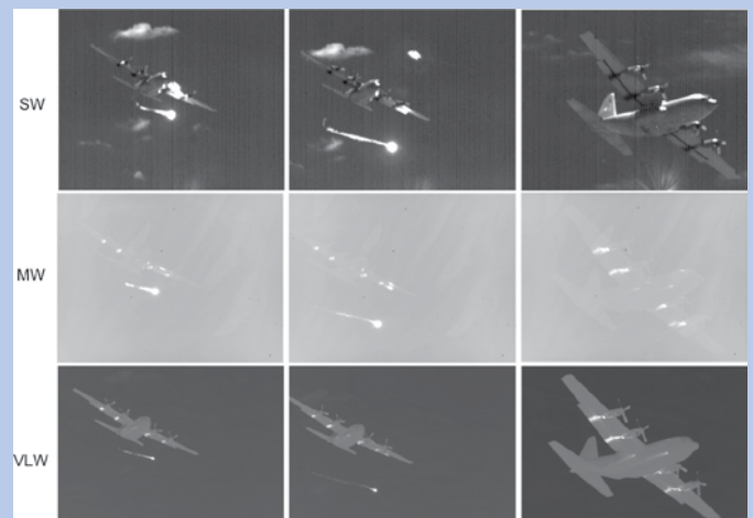
Infrared images of a C-130 Aircraft in the three different infrared bands: short wave (top), medium wave (middle) and long wave (bottom) depicting the contributions made to the aircraft signature within the various bands. These images were captured using imaging radiometers.
