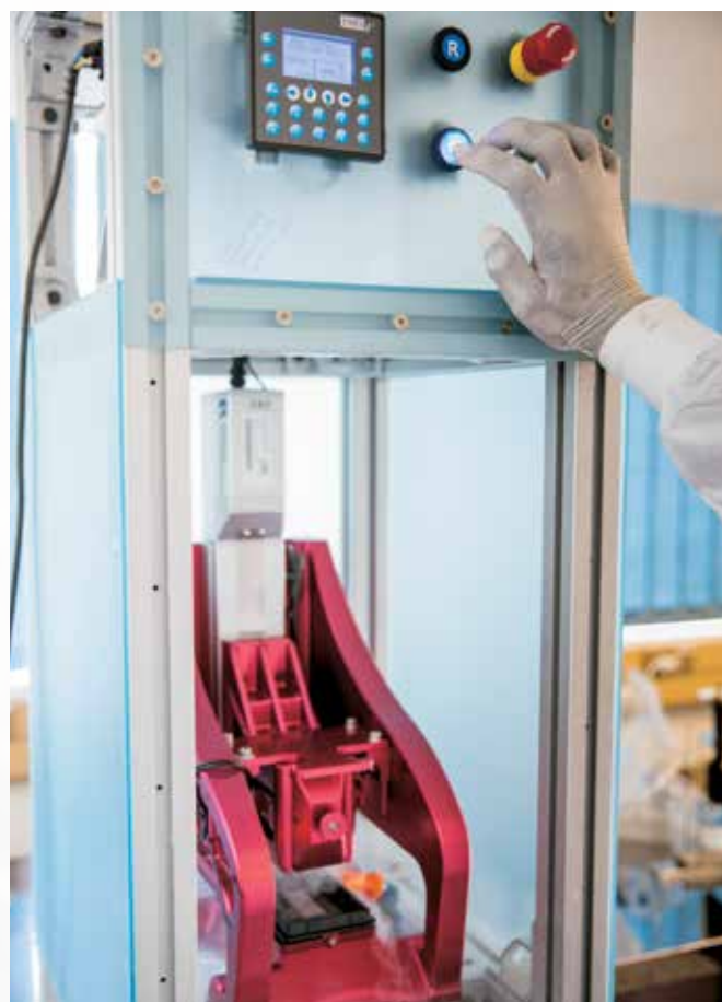
A CSIR researcher using high-throughput microarray printing technology to compress an RNAi experiment onto a glass slide.
