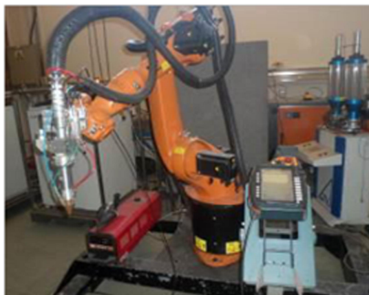
Figure 1. Laser Metal deposition machine set-up
