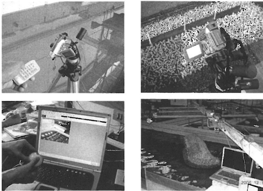
Figure 1. Remote controlled digital video camera or on-line Laptop PC for data capture.
