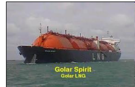
FSRU typically with a capacity of 100 to 170 tcm storage (LNG) and 7 mcm/d (gas) regasification
