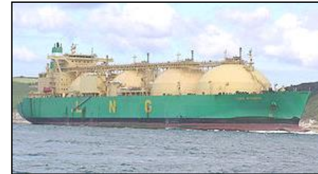
LNG carrier typically with a capacity of 100 to 140 tcm (LNG)
