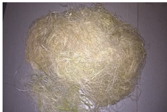
Fig.2. Calotropis gigantea fiber after mercerization
