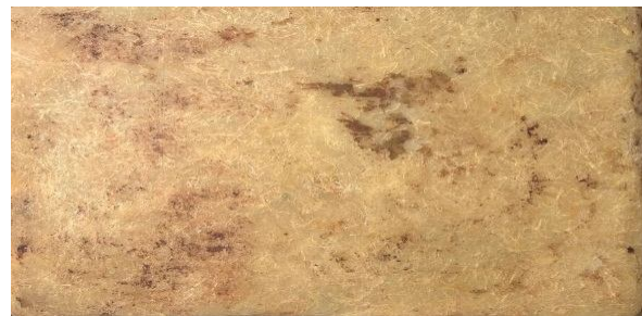
Fig.3. Calotropis gigantea stem fiber reinforced composite plate
