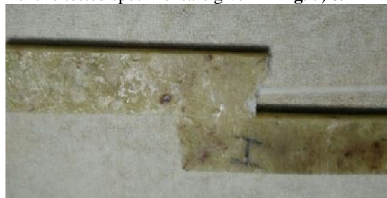
Fig.5. Tensile tested composite sample-12
