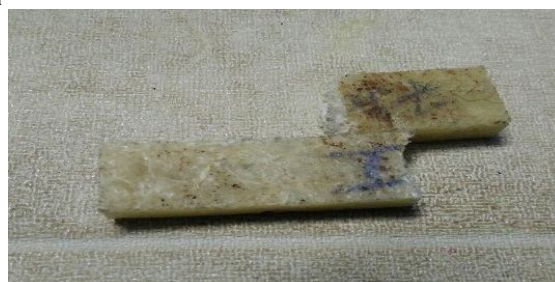
Fig.7. Impact tested composite sample - 6
