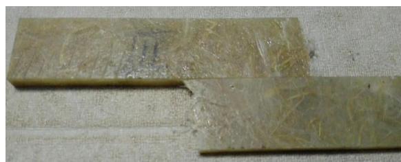
Fig.6. Tensile tested composite sample - 10
