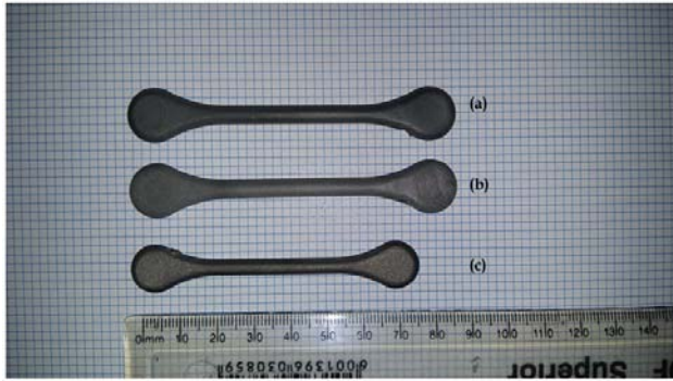
Figure 2—MIM parts of 17-4 PH stainless steel showing shrinkage differentiation: (a) as-moulded, (b) solvent-debound, (c) sintered
