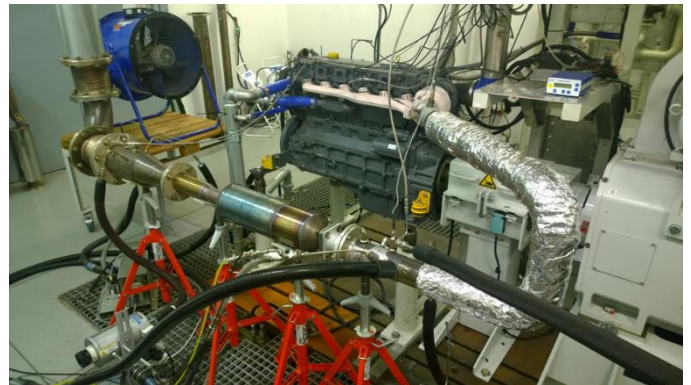
Figure 1. SMF-CRT diesel particulate filter fitted to the engine in a test cell at the Sasol Fuels Application Centre.
