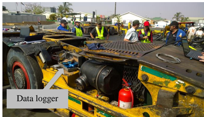
Figure 3. Data logger mounting position on LHD at Bathopele mine in Rustenburg
