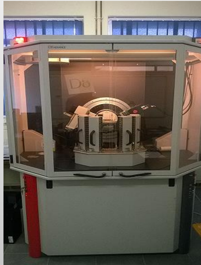
Fig 2: D8-Bruker X-ray Powder Diffraction instrument fitted with a Lynxeye detector (used for XRD analysis)
