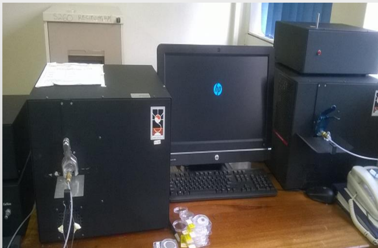
Fig 3: A Thermo-Optical Analyzer (DPM) instrument with an FID detector used for DPM analysis
