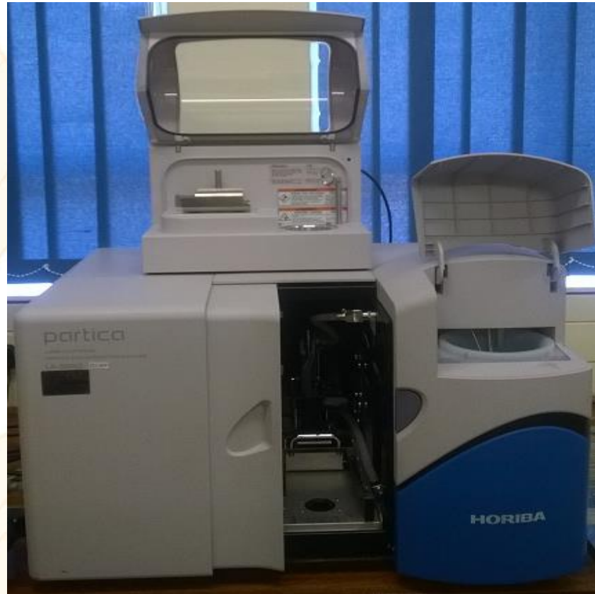
Fig 1: An LA950V2 Laser Light Scattering Particle Size Analyzer used for PSD analysis
