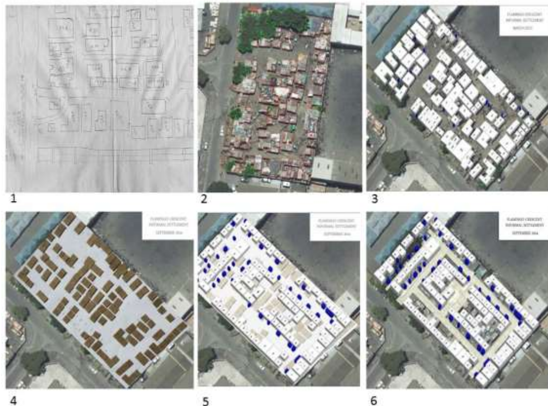
Plate 3: Flamingo Heights Re-Blocking (1) Community drawn map, (2) Digitised from aerial photography, (3) Accurately surveyed and measured 3D plan, (4) Cardboard cuttings – proposed community layout, (5) Re-blocked layout superimposed over community layout - 4, (6) Re-constructed layout (as-built).
