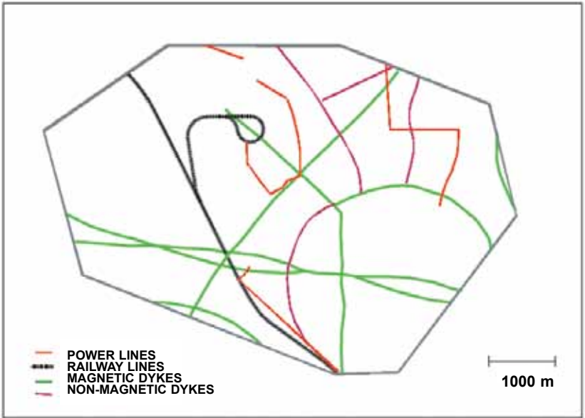
Figure 5.12 Schematic of Dighem survey area showing the major infrastructure and the location of magnetic and non-magnetic dykes 76
