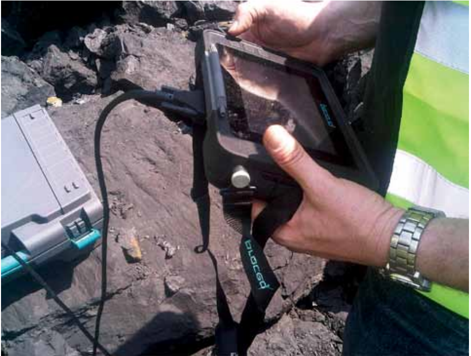
Figure 5.20 Prototype instrument to determine the coal thickness
