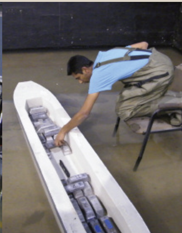
Kishan Tuli loading a model bulk carrier with the right tonnage, at exactly the right spot
