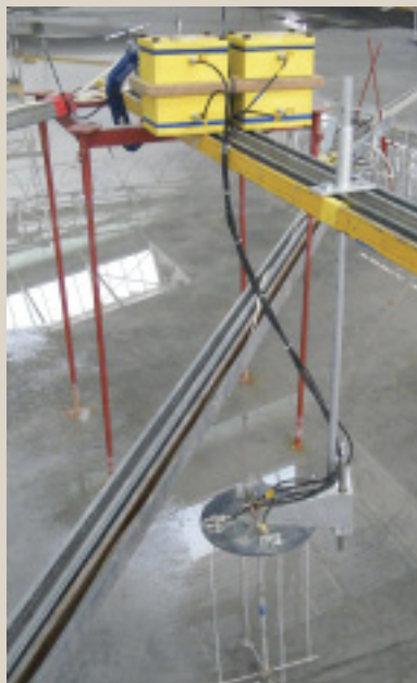
The vessel's movements and reaction to the long waves are monitored closely and recorded by a variety of capacitance probes and keofloats. The keofloat system consists of polystyrene floating blocks monitored with video cameras – these are especially suitable for measuring small and long waves
