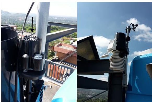
Figure 4. Location of the DAVIS UVR sensor (white dome in the centre of a black housing with small black fins on its rim indicated by the black arrow) on the DAVIS instrument in relation to surrounding physical obstructions.
