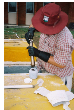
Photograph 5. Expressing cored material into the bottle
