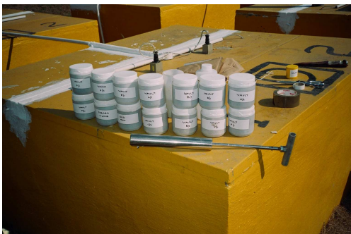
Photograph 4. Coring device and sample bottles
