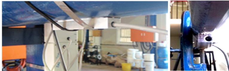
Figure 1: Clamp-on sensors at the 150 mm PCCE and the 40 mm CSIR test loops
