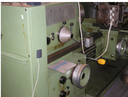
Figure 10: Lathe with RF reader attached.
