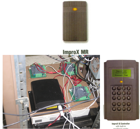
Figure 6: RF tag reader system adapted from a home security system as an Indoor Positioning System (IPS) ( www.aperfectpicklocksmiths.ca )
