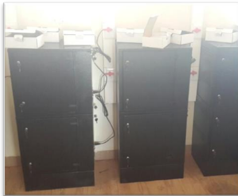
Photo 1-4: Secure charging station used in Phase 2
