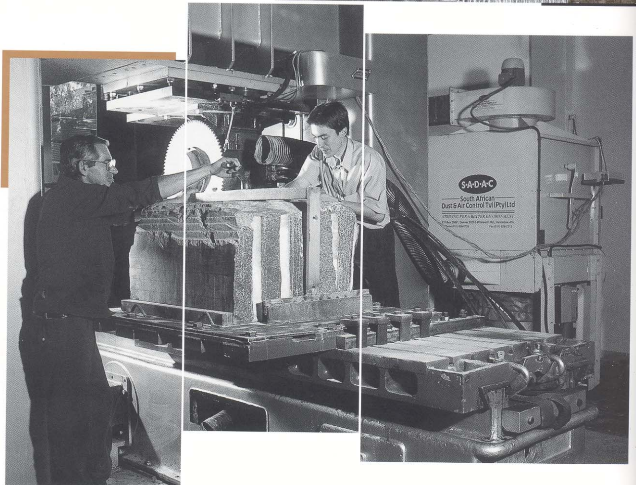
The CSIR is testing an activated saw cutter, a device used by the mining industry, which superimposes vibrations onto a conventional cutting action resulting in lower cutting forces and power requirements. It is suitable for cutting hard rock with conventional tungsten carbide saw tips.
