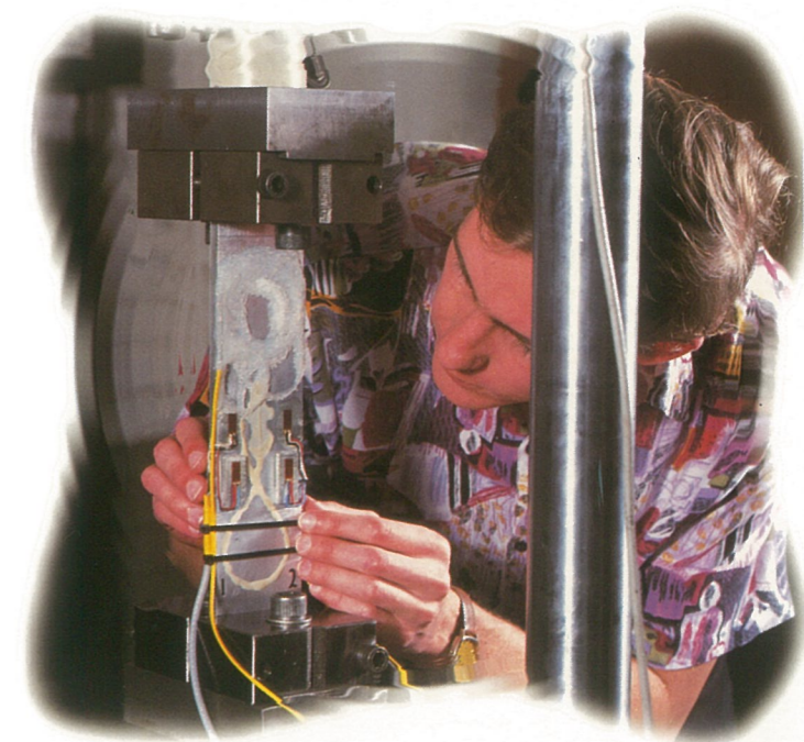
A multiplexed fibre optic strain sensing system has been developed at the CSIR to measure strain on aircraft, and the technology can be customised for many other applications.
