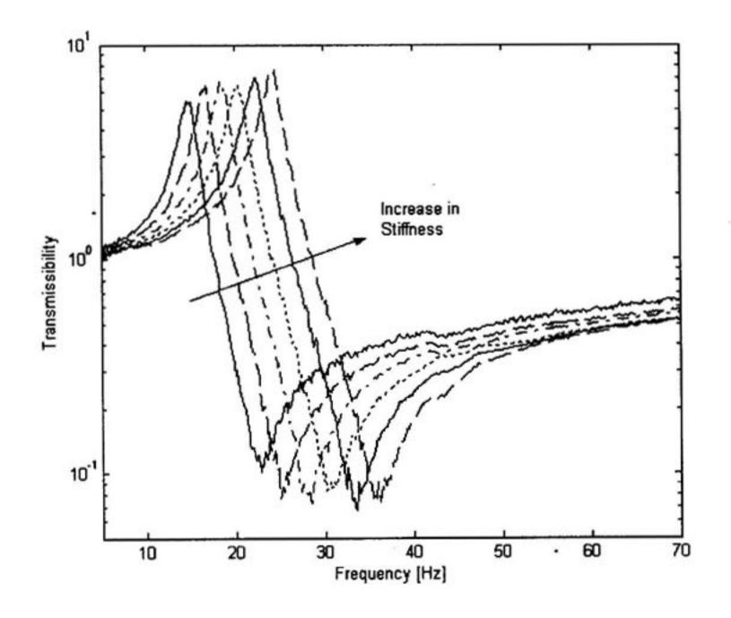
Figure 8. Transmissibility curves for different stiffness values.
