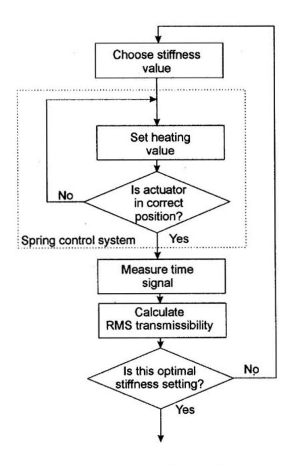
Figure 10. Block diagram of the optimization control system.
