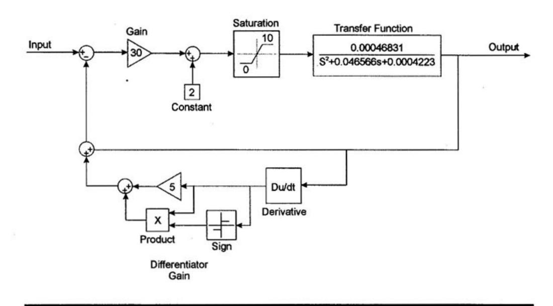
Figure 5. Block diagram of the closed-loop system.
