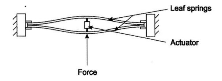
Figure 2. Basic configuration of compound leaf spring.
