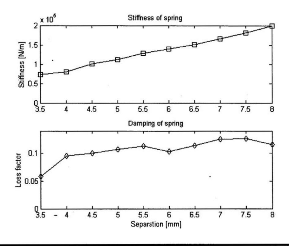
Figure 6. Stiffness and damping of the spring.
