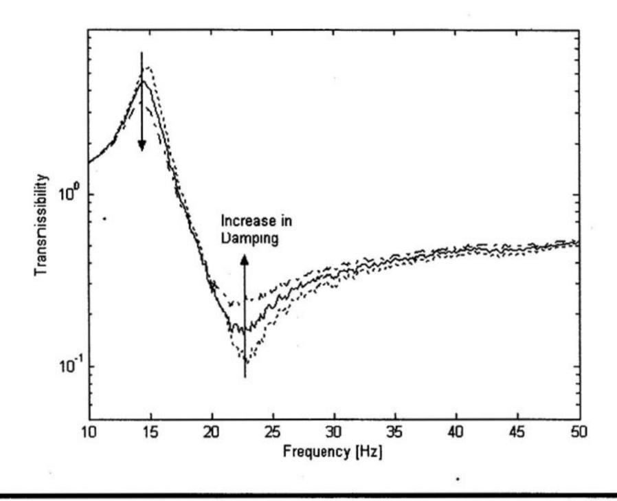
Figure 9. Transmissibility curves for different damping values.
