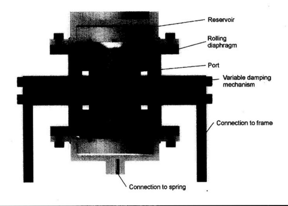
Figure 7. Design of the experimental isolator.
