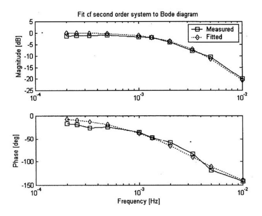
Figure 4. Bode diagram of the open-loop system.
