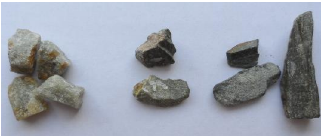
Figure 2: Examples of quartzite aggregate (left), green shale (centre) and grey shale (right)
