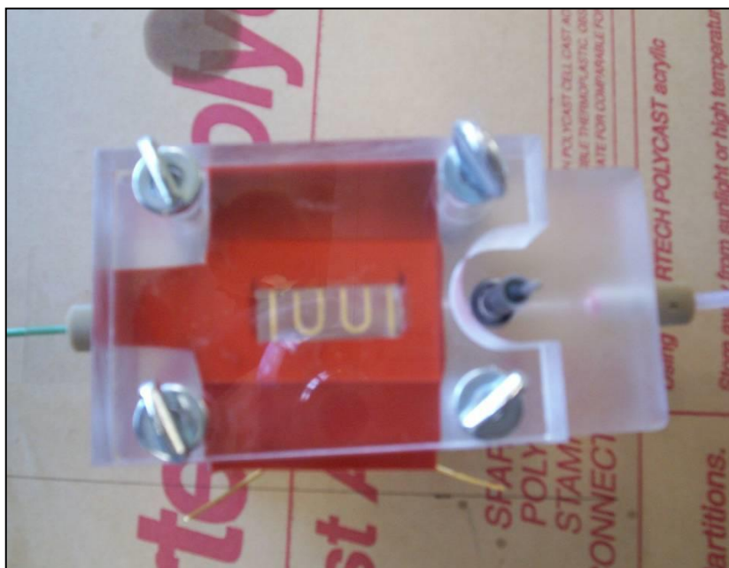
Figure 3.4: Photograph of the electrochemical flow-cell used for Pt deposition (Mkwizu, Modibedi, & Mathe, 2011)
