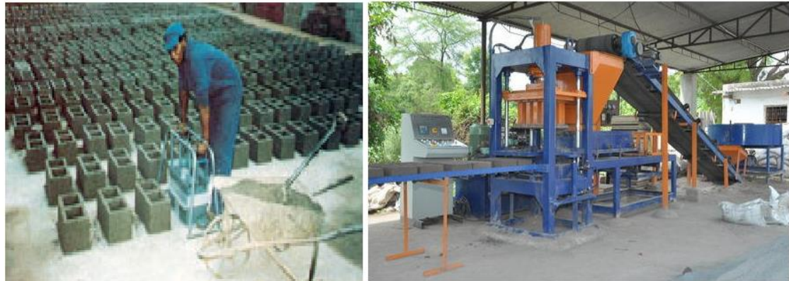
Figure 5: Concrete provides flexibility for manufacturing; the figure shows two manufacturing scenarios, one that is highly mechanised and one that is labour intensive.
