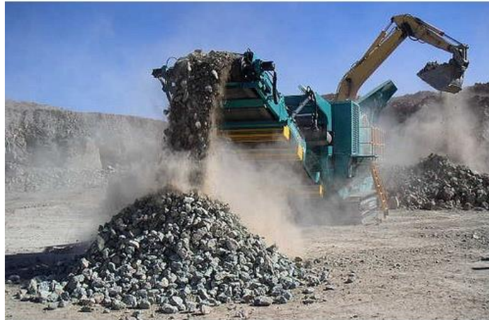
Figure 6: Aggregate being crushed
