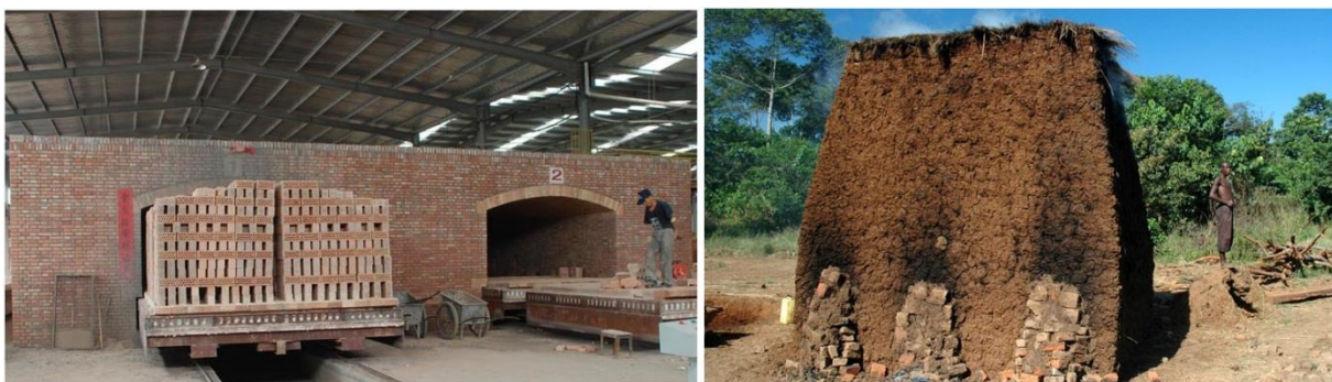
Figure 1: Clay brick processing can be highly mechanised as seen in the first image (left), the image on the right shows the simplicity of the process, with bricks being processed in a rudimentary kiln.
