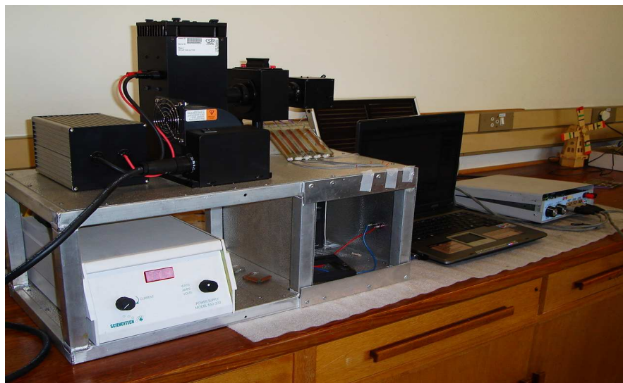
Figure 2.5: A photograph of a solar simulator system used to test cell efficiency
