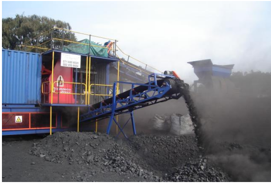
Figure 2: XRT Sorter in operation at Arnot Colliery
