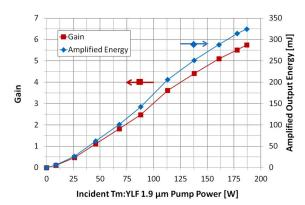
Fig. 3. (Color online) Amplified output energy (right axis) and gain (left axis) as functions of incident 1890 nm Tm:YLF pump power.
