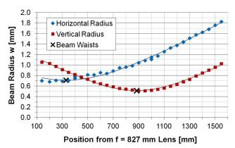
Fig. 5. (Color online) Horizontal and vertical second moment beam radii as functions of distance from an f = 827 mm lens combination at maximum output at 50 Hz. The lines are fits of the beam propagation equation to the measured data and the crosses are the fitted beam waists.
