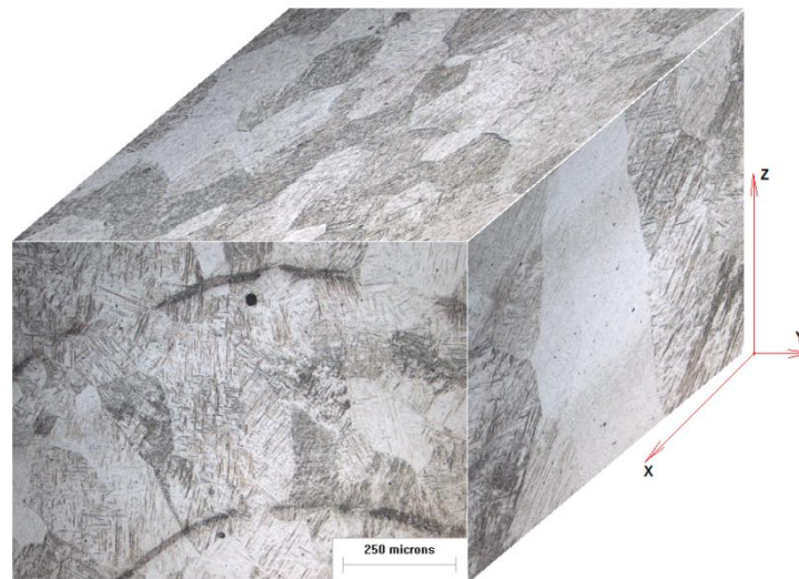
Figure 7. Typical grain structure, of the LAM Ti6Al4V component, shown in 3D
