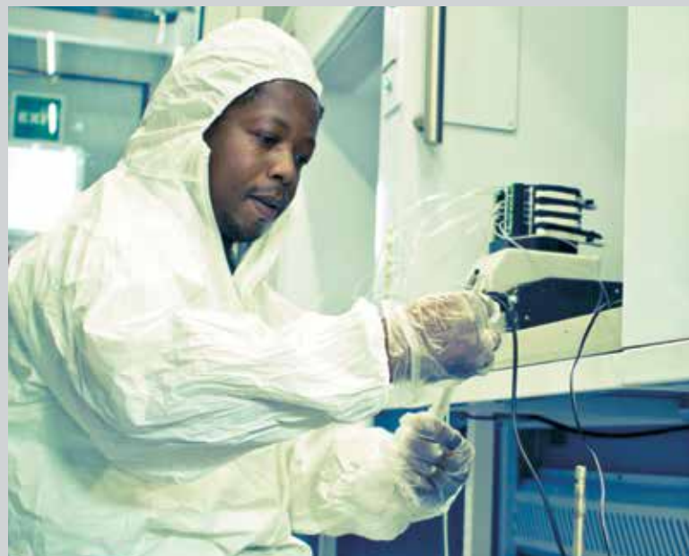
CSIR researcher Dr Thato Mtshali analysing the iron concentration in a seawater sample.
