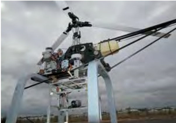
A 125cc helicopter platform to monitor electricity transmission lines.
