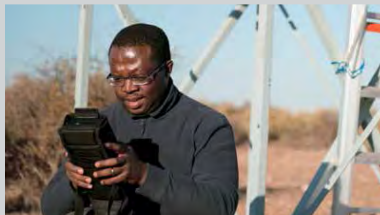
A sun photometer is used to measure aerosol optical thickness and precipitable water vapour.
