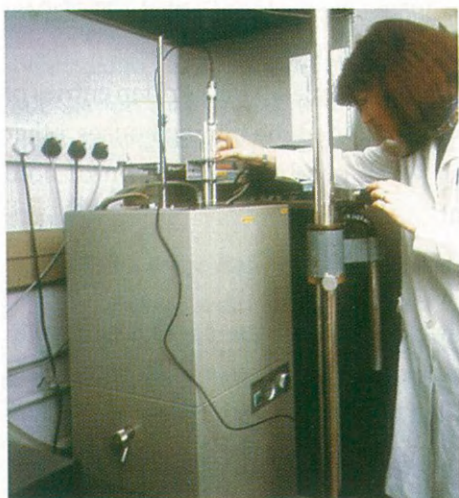
Constant temperature bath for calibrating mercury in glass thermometers
