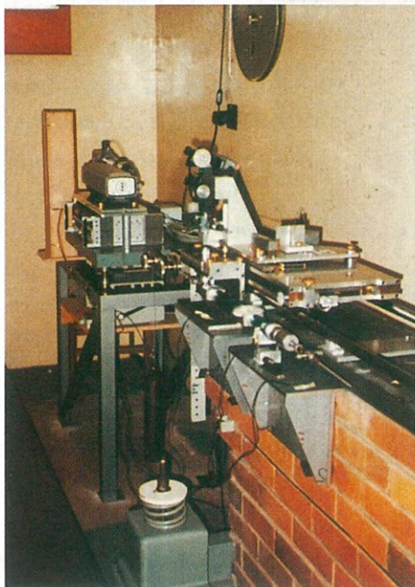
Equipment set up in the tape tunnel to measure the positioning wires for the National Accelerator Centre
