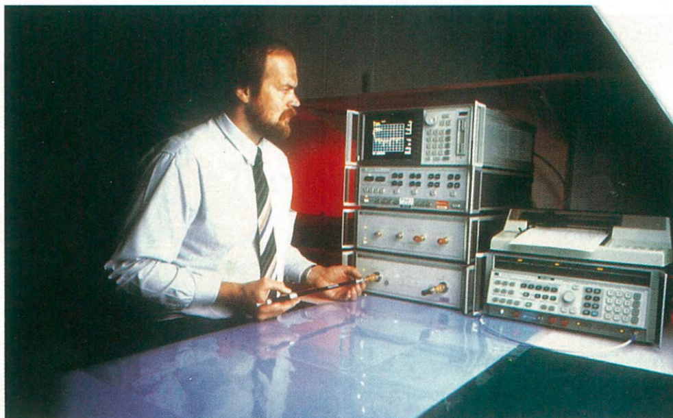
Eric Dressler calibrating the vector network analysis system, 1996
