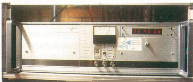
Caesium time and frequency standard
