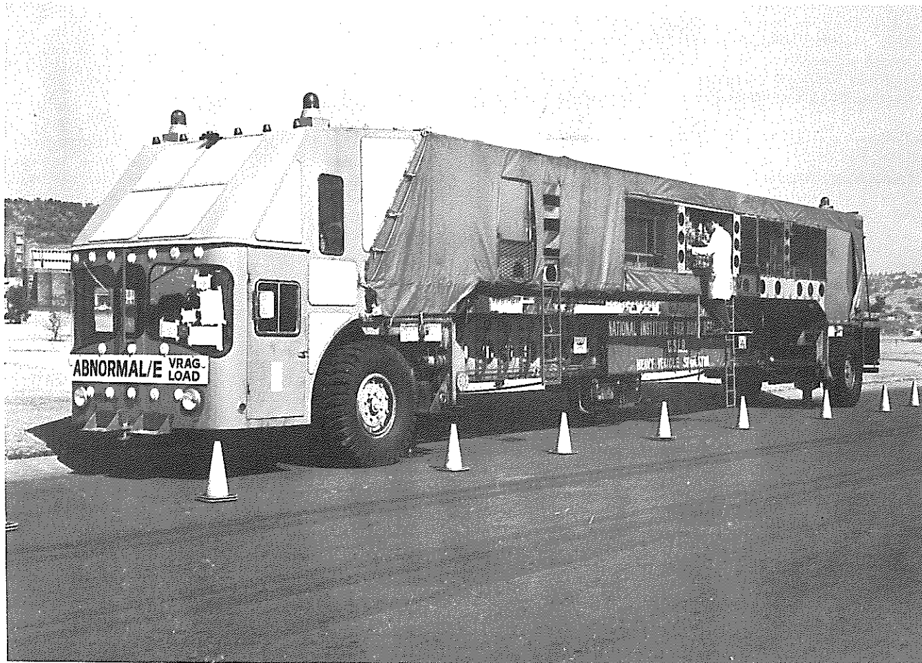
The NIRR heavy vehicle simulator.
