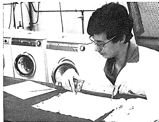
Measuring area shrinkage of samples after machine washing.
