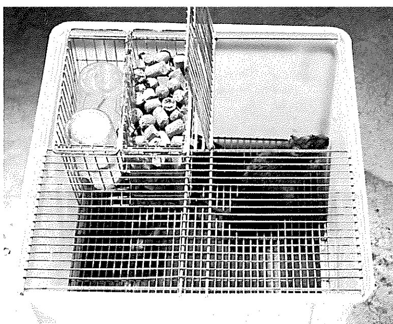
The improved metabolism cage developed by the National Nutrition Research Institute for biological determination of protein digestibility using experimental animals
