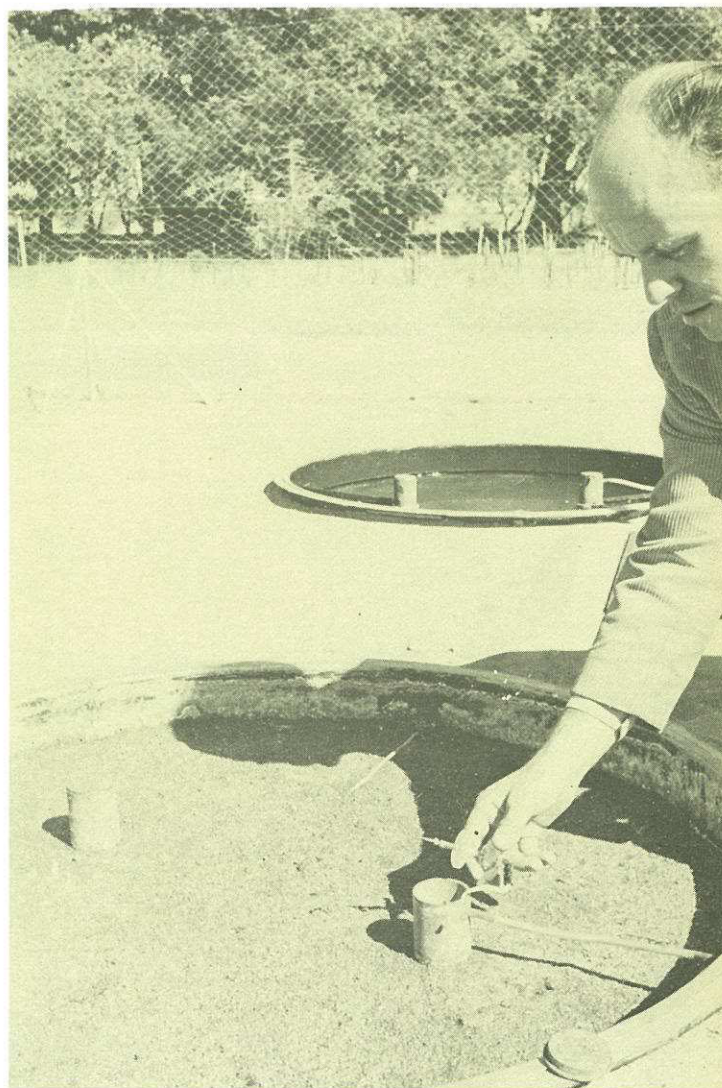
Research into the influence of evaporation on water salinification is carried out with the aid of these underground tanks at Gross Barmen in South West Africa.
