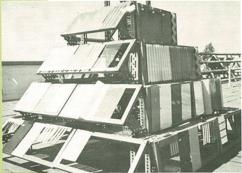
Exposure tests on various plastics and related materials that are being offered for use in building
