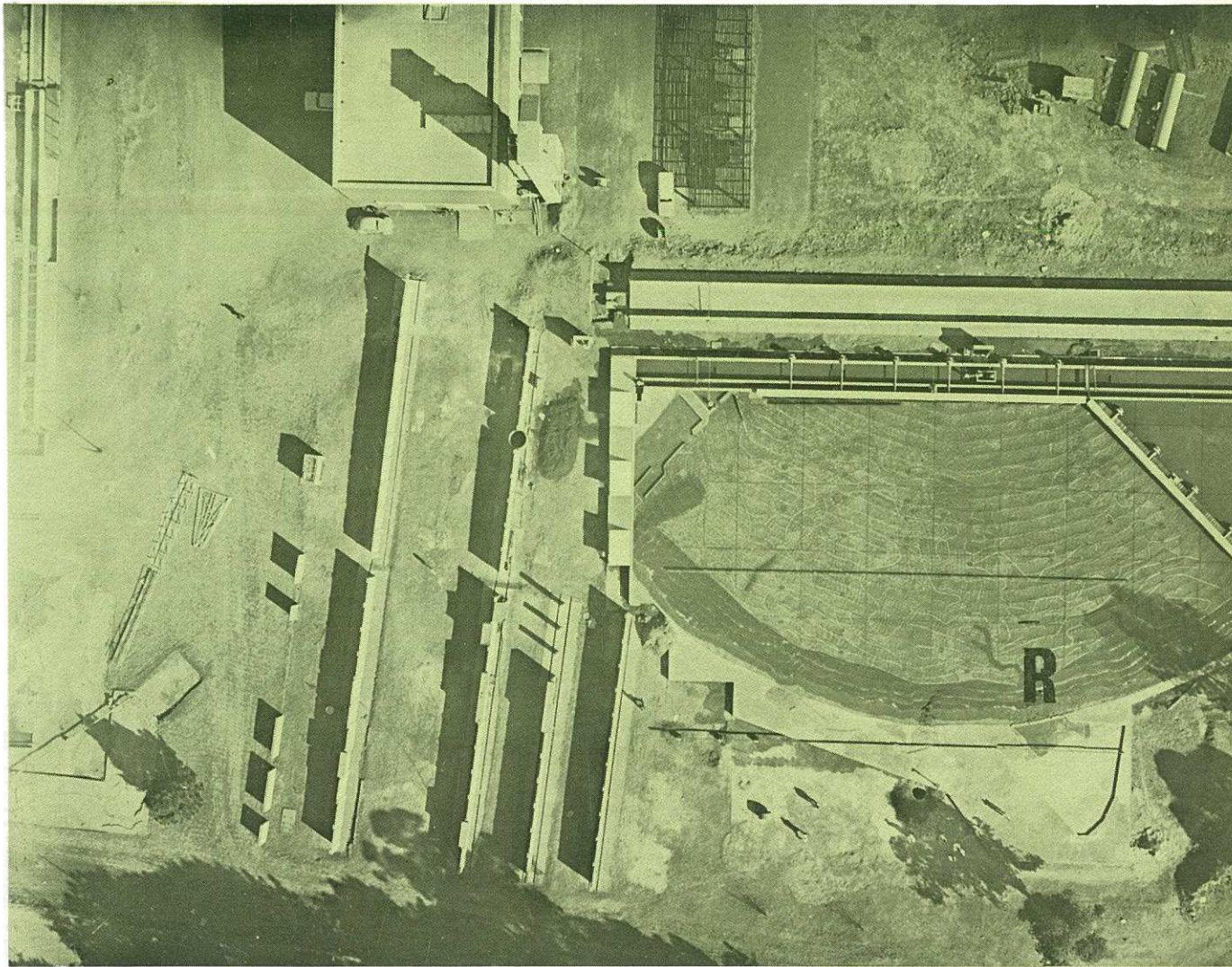
A model of Table Bay harbour on the CSIR site in Pretoria showing the location of the proposed fishing harbour at Rietvlei (marked 'R')
