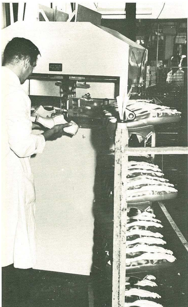
A heat setter designed by LIRI in operation in a South African footwear factory
