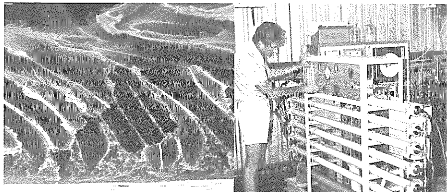
This small reverse osmosis plant, which utilises spiral-wound membrane modules contained within the pipe-like pressure vessels, delivers 5,8 m 3 of drinking water per day (bottom right).
