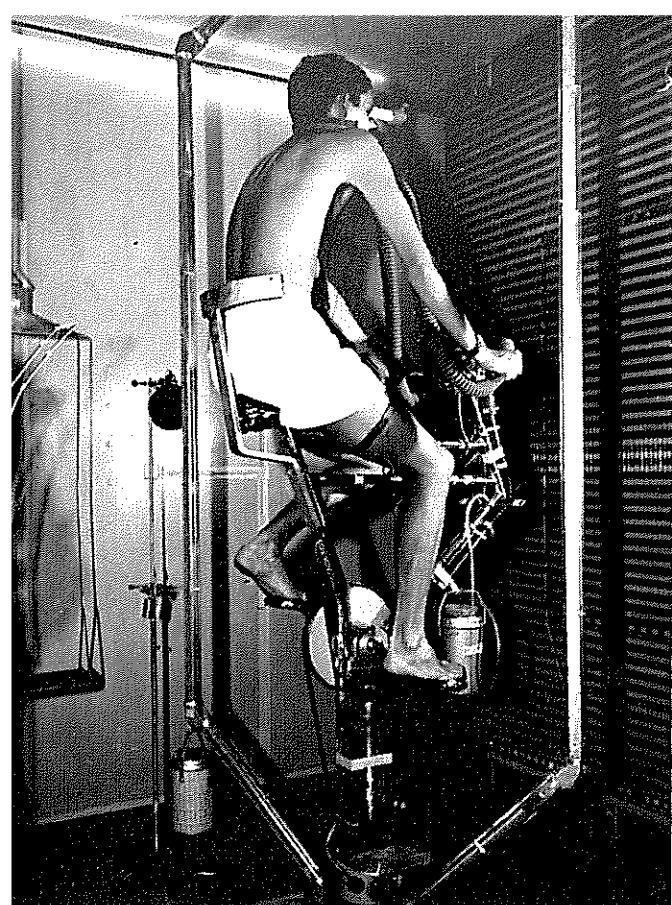
The heat exchange between a test person and his environment is measured in the Chamber of Mines' climatic chamber. The climatic chamber and the apparatus were designed by the CSIR.
