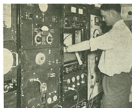
A mobile acoustics laboratory for field work on problems such as the acoustics of studios, halls, cinemas, etc., transmission of noise in buildings and the reduction of industrial noise. Tests are made with electronic equipment in the mobile laboratory, which is connected by cable to microphones, loudspeakers and other apparatus set up in the building under test.
