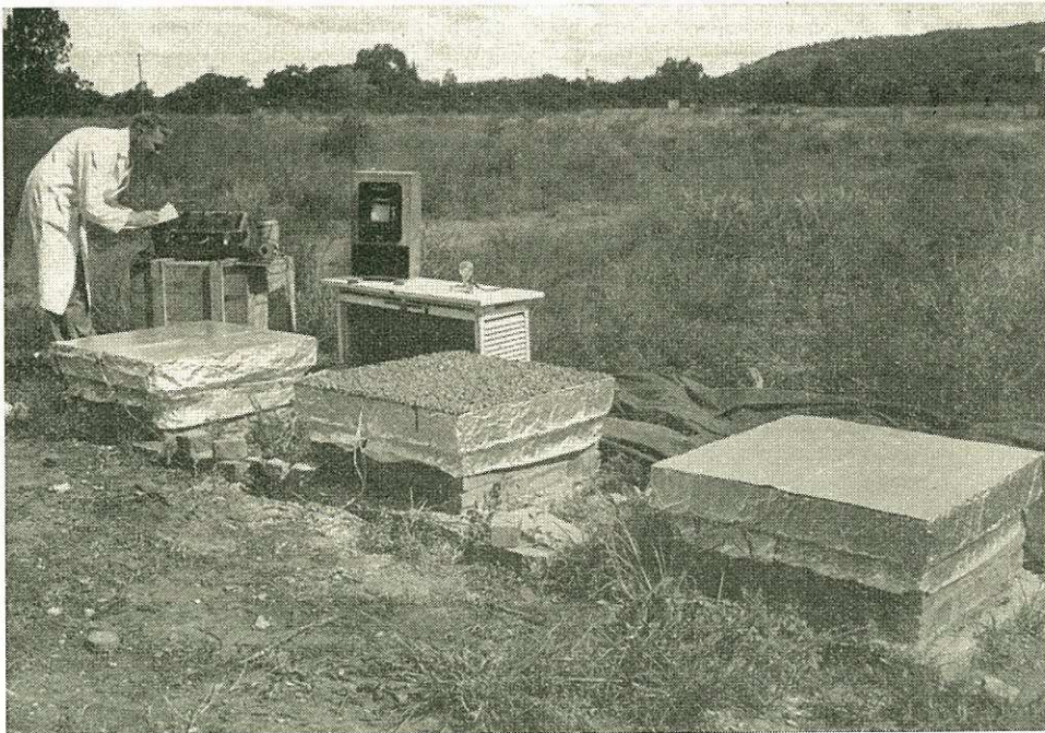
A comparative test to determine the protection against solar heat afforded by a concrete slab covered with various roofing materials.
