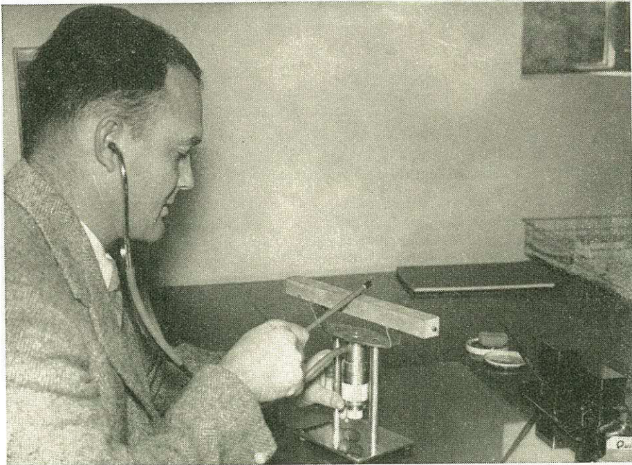
The deterioration of a concrete sample by corrosion can be determined by measuring its elastic properties with this audio-elasticity meter invented in the Acoustics Section of the N.P.L.
