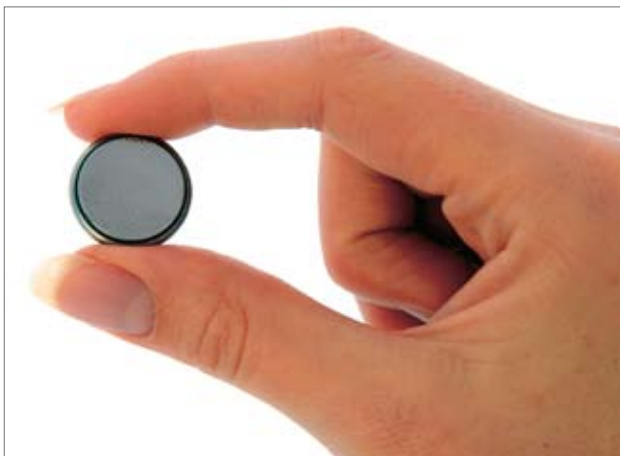
Coin cells are basic battery cells that researchers use to test changes made to its cathode chemistry.
