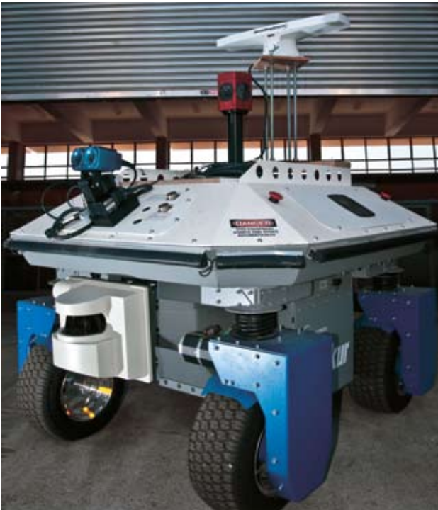
The rover is being used as the base platform in the Mule project. CSIR researchers have integrated cameras, laser scanners and GPS modules to enable it to perceive its environment.
