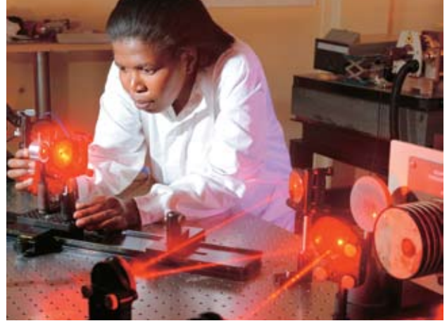
A CSIR researcher aligns a laser as part of a laser-based heating system for diamonds.
