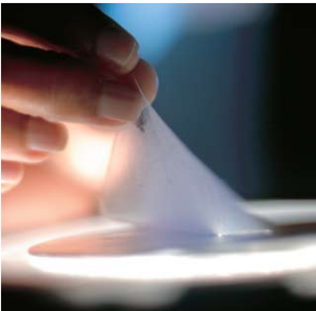
Electrospun chitosan nanofibres that have been found to have certain antibacterial properties.
