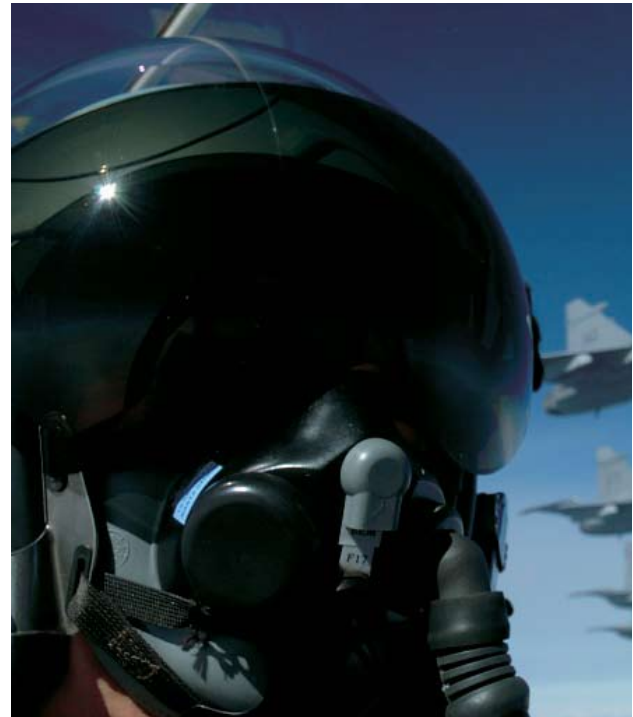
The Cobra helmet, as used in the SAAF's Gripens, can display critical data onto the visor and tracks where the pilot is looking. Images copyright Gripen International.
