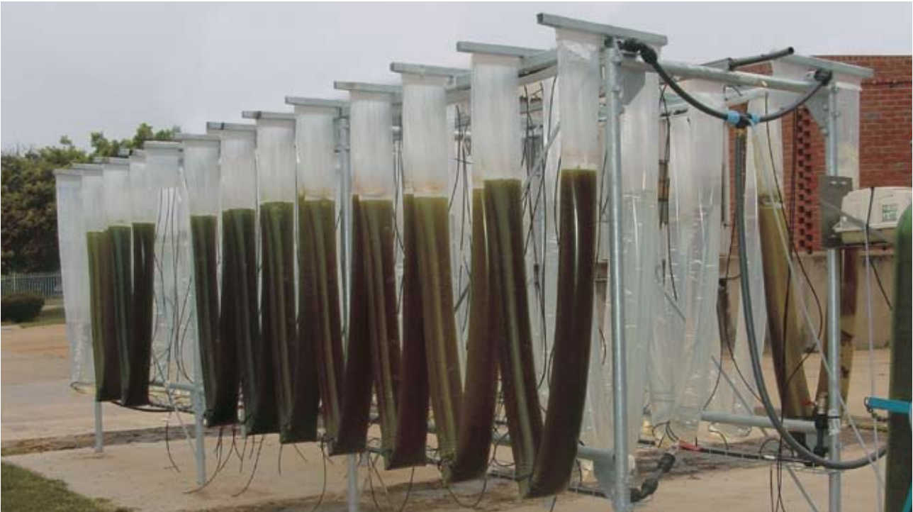
A pilot scale photobioreactor at the CSIR Modderfontein campus containing an algal species that has demonstrated good potential as a biodiesel producer.
