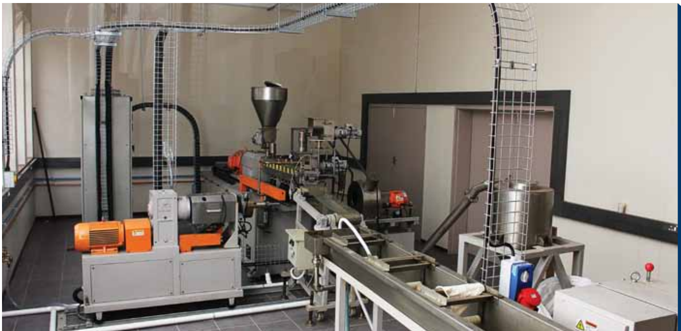
The newly-acquired, industry-scale extruder at the National Centre for Nano-Structured Materials is a machine which is normally used for melting a plastic polymer and then converting it to a certain shape through a process called extrusion. The extruder can be used to mix the polymer with additives or nanostructured materials to prepare a polymer nanocomposite in order to enhance the properties of the polymer such as fire retardance performance.
