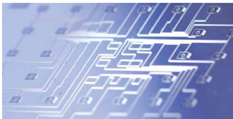
A typical microfluidic mould used for the manufacturing of devices.
