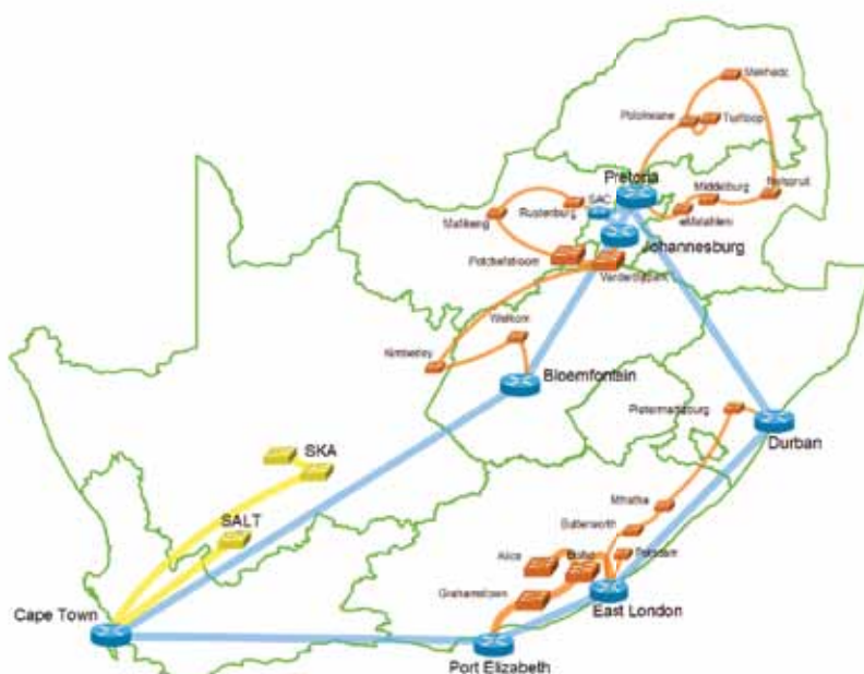
A map showing the SANReN national backbone in blue. Yellow lines indicate extensions under completion. The orange lines indicate future backbone extensions.
