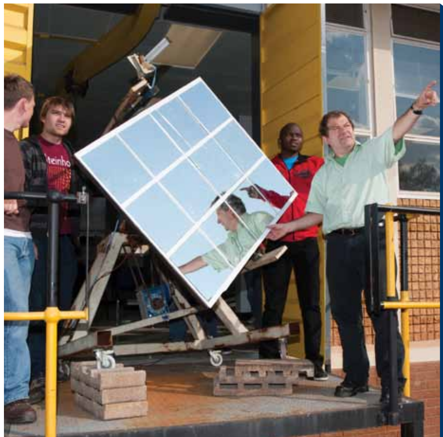
A mini-heliostat was installed to check the tracking and control system. Pointing to where the focal beam that is reflected from this single heliostat is concentrated, is Thomas Roos with students from the universities of Stellenbosch and Johannesburg.
