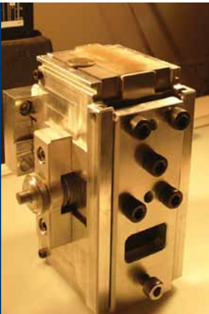
The printing head used to print experiments on glass wafers.
