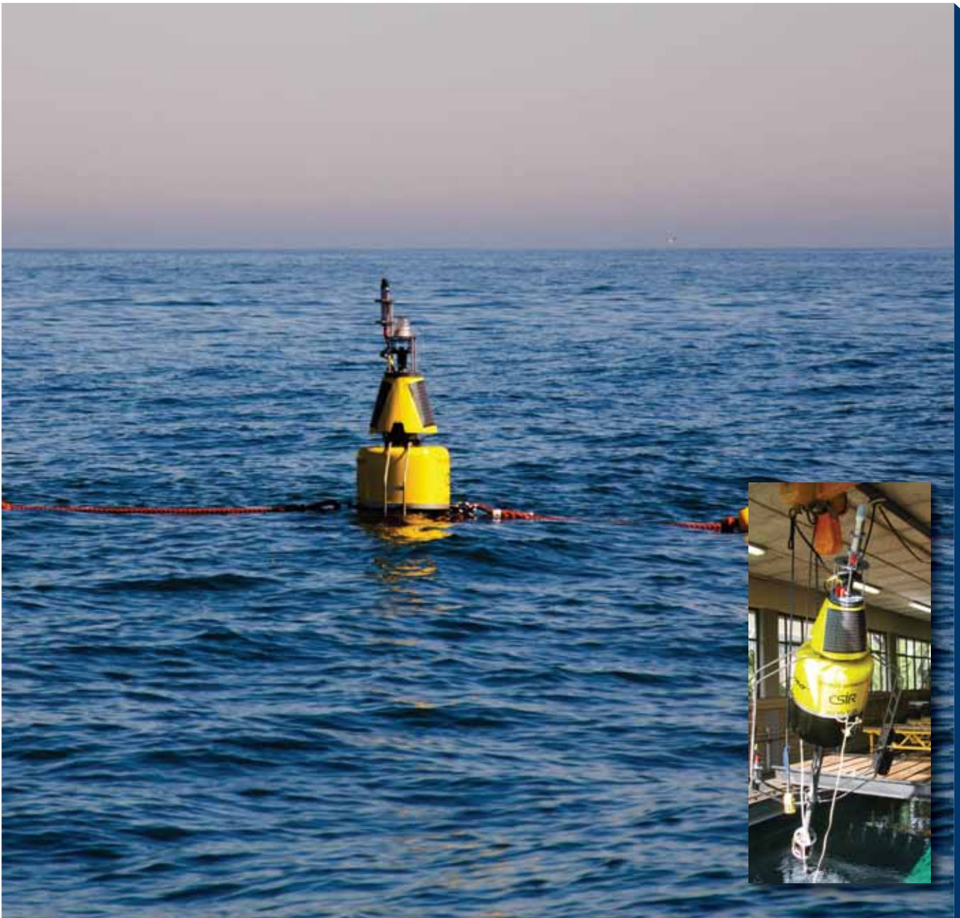
As part of the CSIR's Safe Water Earth Observation Systems project, researchers developed a low-cost, low-weight pencil-buoy that is easy and fast to deploy. It will also soon feature new low-cost radiometric sensors, also developed by the CSIR. These new buoys will be used to provide real-time data on algal blooms. They will also verify new satellite techniques, which will then allow satellite data records from 10 years or longer to be used to characterise change in South African coastal and inland ecosystems.
