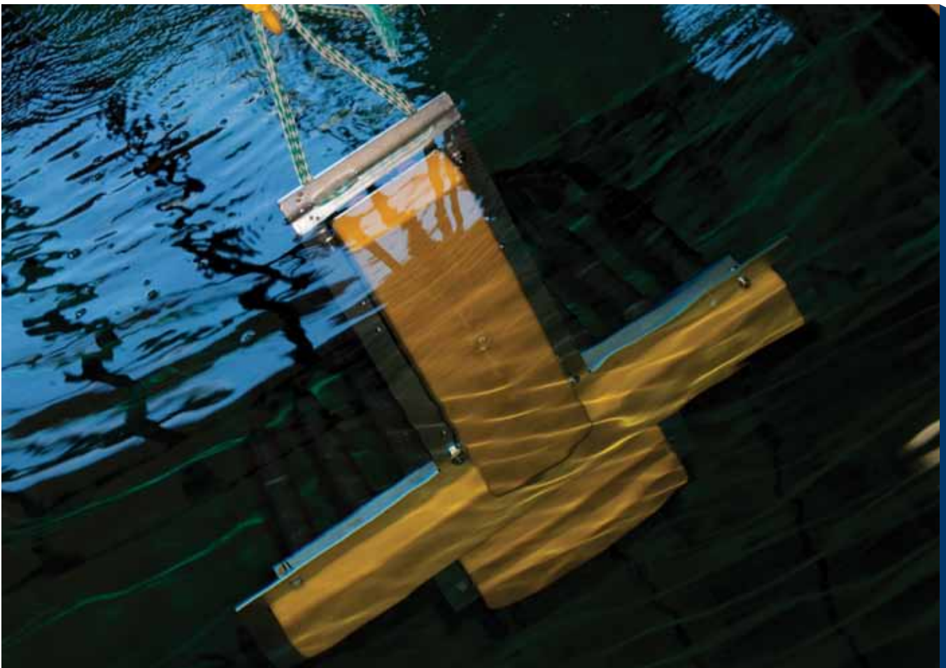
Prototype 3D imaging array showing the high acoustic bandwidth transmitter (vertical) and receiver (horizontal) arrays for producing 3D underwater images.
