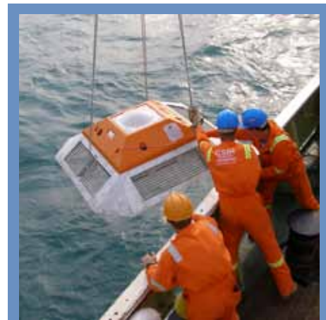
The CSIR team deploying an anti-trawl mooring in the ocean.
