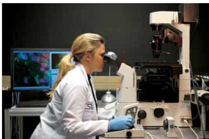
Dr Janine Scholefield imaging induced pluripotent stem cells on a custom-built, super-resolution PALM/STORM microscope, built by the CSIR's Dr Musa Mhlanga and former PhD student Dr Ricardo Henriques.
