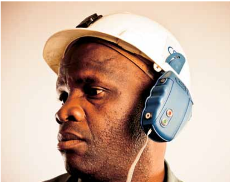
A miner wearing the CSIR safety device used in the detection of loose rocks overhead.
