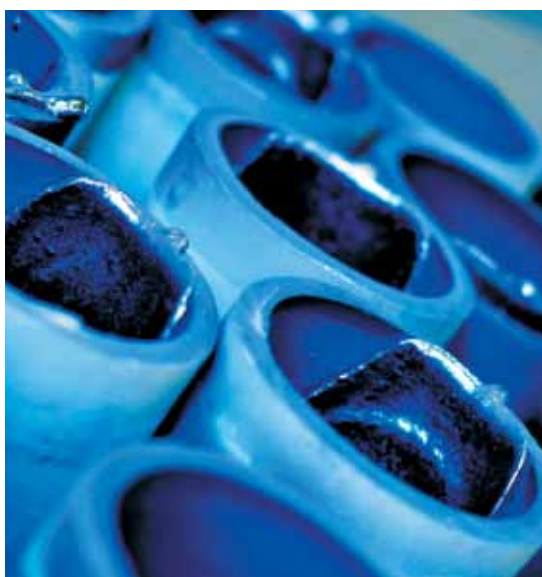
Cups in which titanium had been melted in a vacuum furnace during the investment casting process are featured above. Pictured top right is a sample of the titanium powder produced using the CSIR's process.
