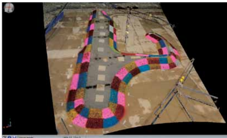
A picture-perfect view of the 3D laser scanner's ability to extract colour as well as coordinates of a surrounding area of interest for an Australian project, within seconds of acquisition; compared to a photo of the scanned area (below, left).
