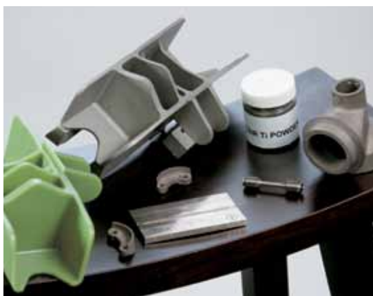
Samples of parts manufactured from titanium powder through two different manufacturing methods, namely powder metallurgy and investment casting. Also shown is the wax part from which a cast will be made for the investment casting process.
