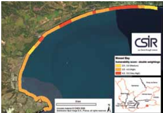
CSIR coastal engineers used a coastal hazard risk model to develop a spatial assessment that combined a broad set of drivers of sea-storm risk along the Mossel Bay to Glentana coast. The following drivers were considered and integrated into an overall 'vulnerability score' for the coastline: elevation, distance to infrastructure, tidal range, maximum offshore wave height, degree of wave protection, historic erosion, geology, geomorphology, ground cover, human actions and relative height of the protective foredune buffer.
