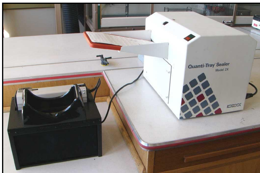
Figure 2.6: Colilert Quanti-Tray sealer and UV light.
