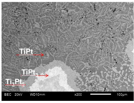
Sintering condition: 1400 ° C\_10mins\_60MPa
