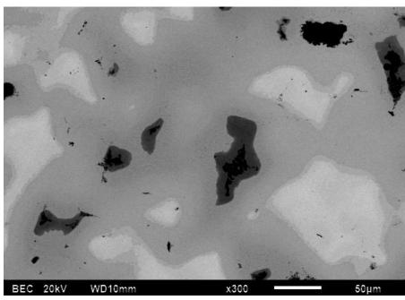
Sintering condition: 1200 ° C\_25mins\_60MPa
