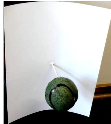
Figure 7: Multi-sensor setup with SR4000 TOF camera, FLIR A300 IR camera and XBOX Kinect rigidly mounted on a tripod (left), and tennis ball calibration object (right)
