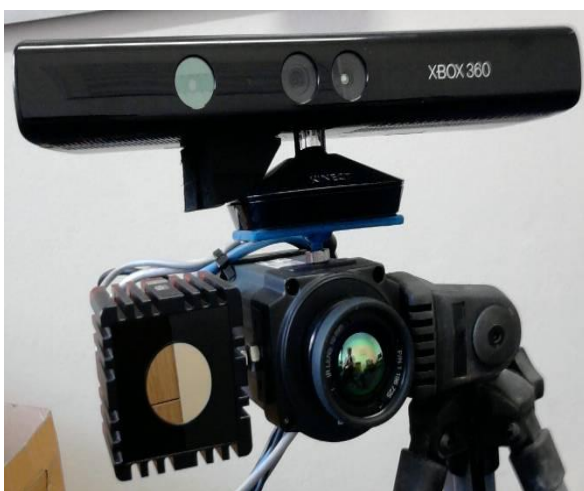
Figure 8: Single-frame alignment fusing XBOX kinect and FLIR A300 IR camera
