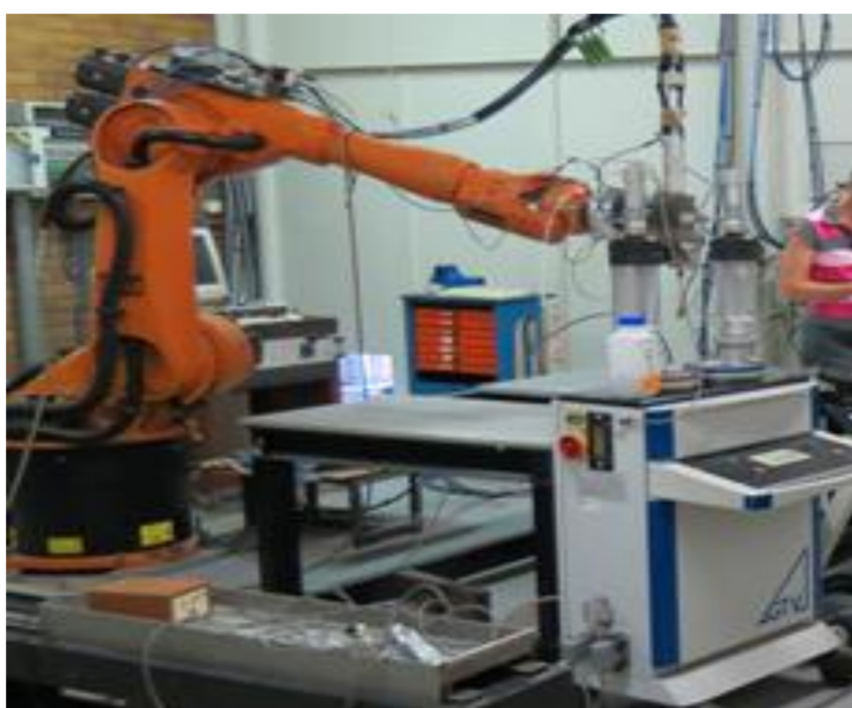
Figure 1: Rofin Nd:YAG laser used for irradiation of the powder on the substrate.
