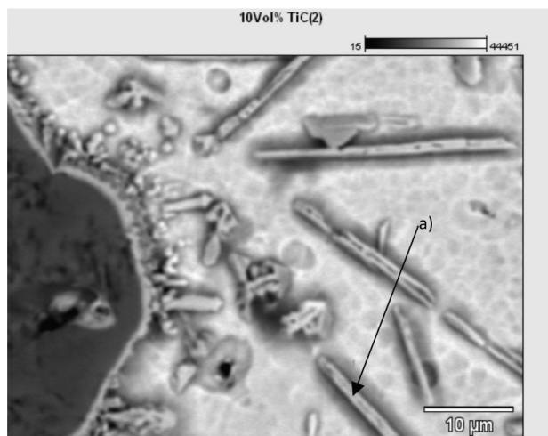
Figure 12—Backscattered SEM micrograph showing decomposition of TiC
