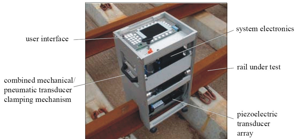
Fig. 2 Inspection system developed at Imperial College and Guided Ultrasonics Ltd (courtesy of Prof. P. Cawley).
