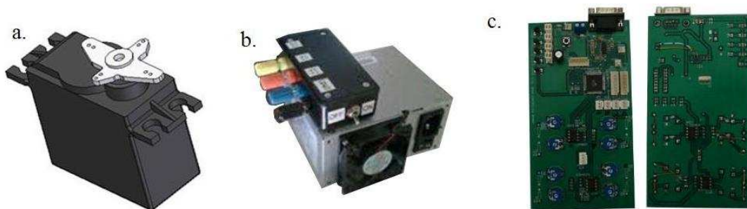
Figure 13 (a) Model helicopter servo motor, (b) Modified PC power supply, and (c) Generic controller board
