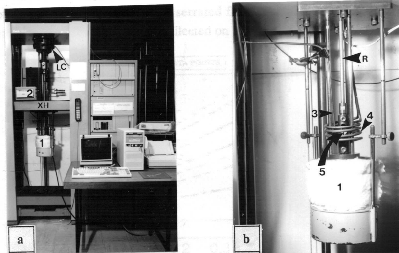
Figure 3.2 (a) Computer-interfaced Zwick 1484 materials tester, with test rig mounted underneath cross-head (XH), showing 200 kN load cell (LC) and temperature controller (2). (b) Close-up view of rig, showing the temperature bath (1) (which has been lowered to show the coil and specimen), chromel-alumel thermocouple (3), heating coil (4) and specimen (5). The specimen is put into tension by the downward force exerted on the bottom end of the specimen by the downward movement of the cross-head and rig, while the top end of the specimen is kept stationary by the restraining rod (R), which is attached to the load cell.
