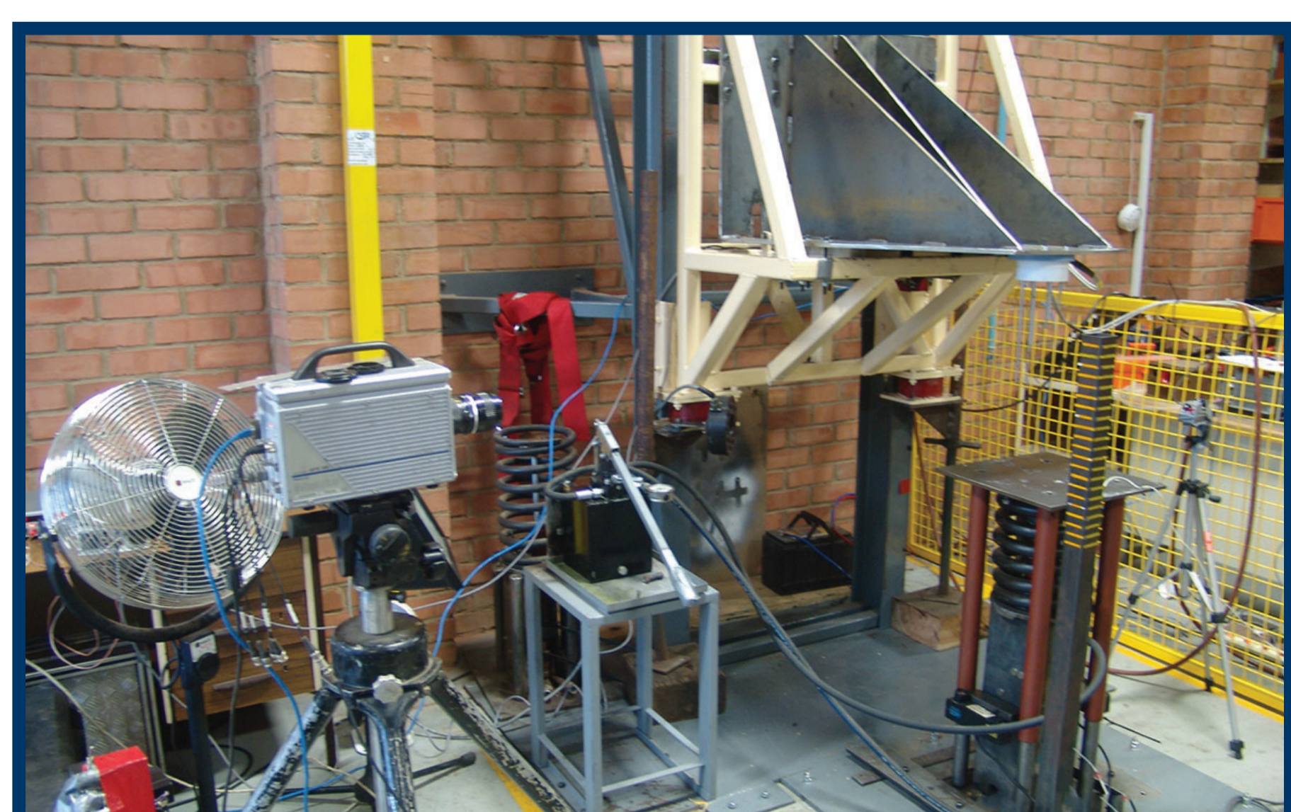
Figure 4: Mechanical Deflection Sensor actual setup
