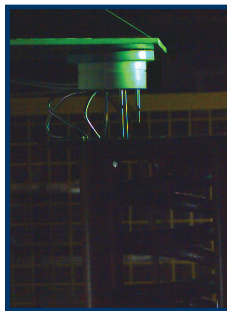
Figure 5: Bending rods of the Mechanical Deflection Sensor
