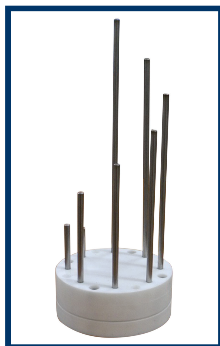
Figure 2: Manufactured Mechanical Deflection Sensor
