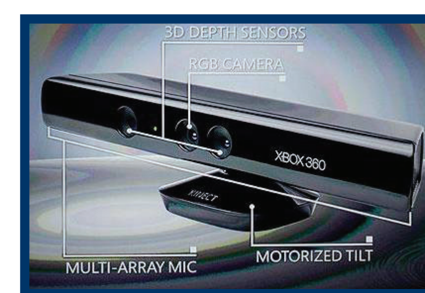
Figure 4: The Microsoft Kinect sensor with its RGB camera and 3D depth sensors [14]
