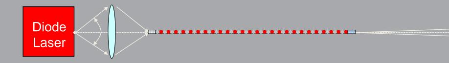
Mode: Continuous Power : very high Beam Quality: very bad Wavelength: TBD Efficiency: 50% Power supply: DC Technology: Semiconductor Size & weight: small Mode: Continuous Power : high Beam Quality: perfect Wavelength: choice Efficiency: 50-80% Cooling required Technology: fibre laser Size & weight: compact
